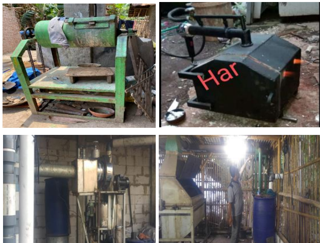
Figure 4 Traditional Machines for Crushing, Smelting, and Filtering Toxic Fumes
